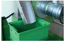
Installation of compressed air nozzles will facilitate the DC-20 cleaning process when light materials have been sorted and cleaned.
